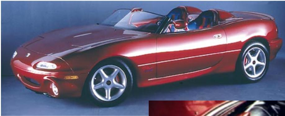
The Miata M-Speedster made its debut at the 1995 Chicago Auto Show. Designed by Wu-Huang Chin of MRA, it featured a 1.8 litre supercharged engine that developed a healthy 200bhp.
