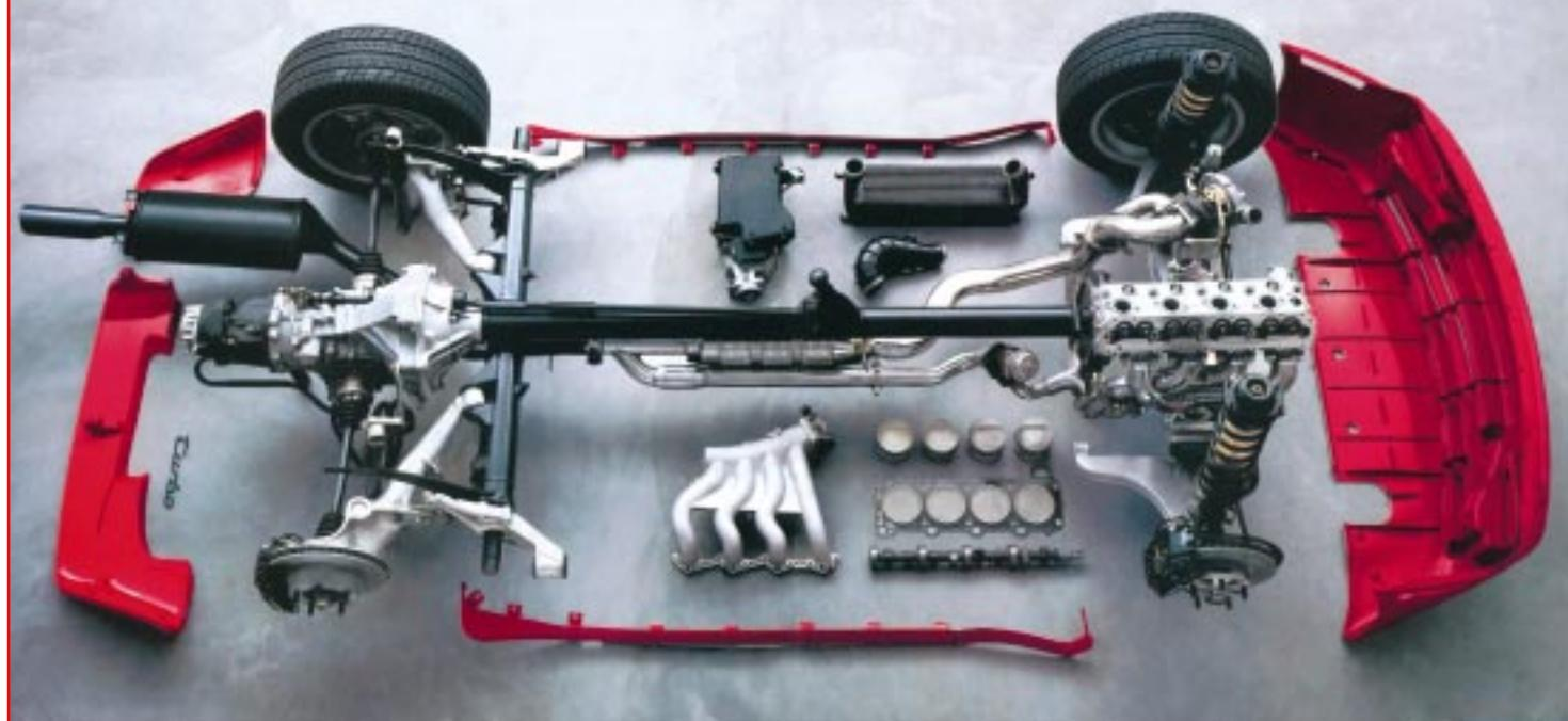
*This superb advert from America shows all the major components used in converting the normally-aspirated 944 to a 944 Turbo. Although developed for the turbocharged model, a number of these parts, such as the cast aluminium alloy suspension pieces, were carried over onto the standard car.*
