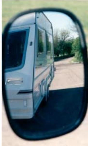
*Almost immediately the tail of the caravan begins to veer to the right. Its image is decreasing in the left mirror (not shown). Correction right hand down on steering wheel.*
