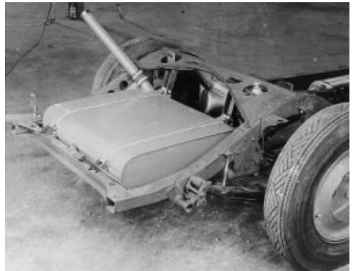
*And so to a detail of the rear of the chassis and fuel tank. Automatic lubrication pipes are in evidence around the springs as are the threaded shackle pins, often considerably worn on neglected cars. See too the absurdly inaccessible fuel filter poking up through the chassis cross member on the right side, and the unusually shaped silencer to the left.*
