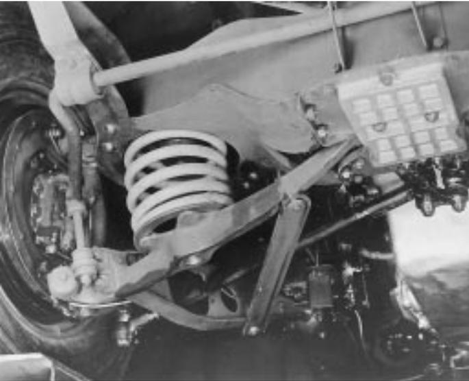
*Now, looking from underneath, all the major suspension and steering components are visible. Note the massive front cross member above the spring and the square jacking pad which was of a different type to that generally used in volume production. The strut between the triangle levers in the middle of the photograph is a brace.*
