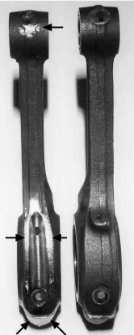
Lightened and balanced 998 connecting rod (left). Shot peened the reworked areas (arrowed).
