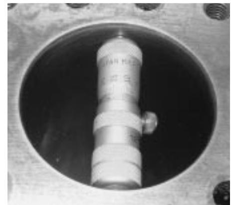
**Measure the bore with an inside micrometer and the piston diameter with an outside micrometer - the difference is the piston to bore clearance.**
