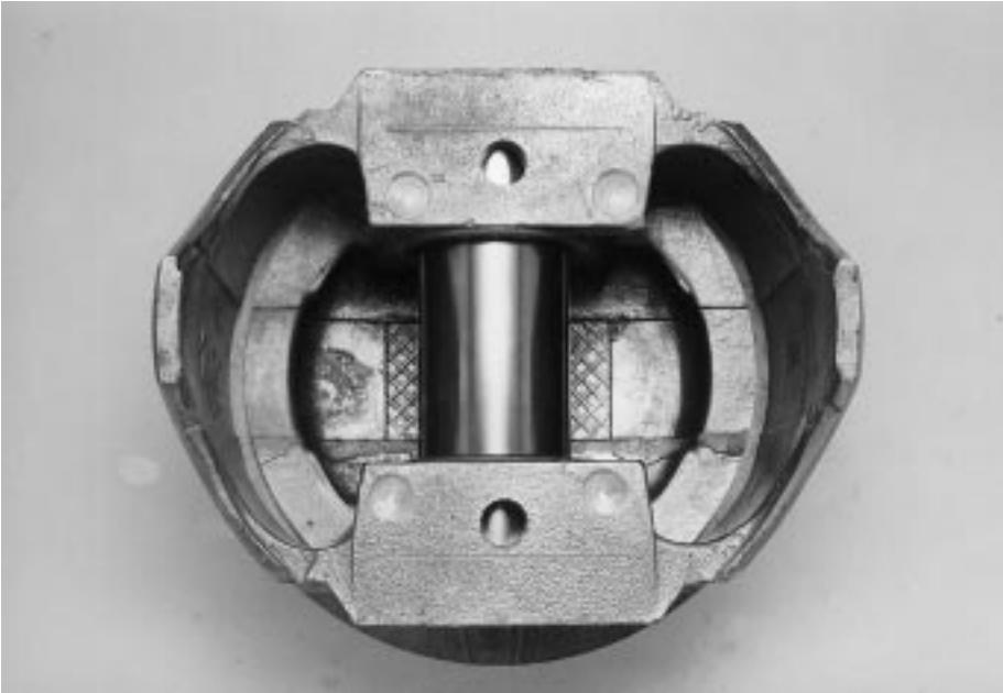
**Underside of an typical cast aluminum piston which does not have a steel strut. This piston will withstand use in an engine which will be revved to 6000rpm for short periods; it will not withstand sustained high rpm use.**
