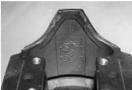
**View of the inside of a piston skirt showing how the edge is made thicker for strength.**
