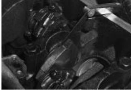
**Feeler gauge being used to check the crankshaft end play (float). Lever the crankshaft forward with a large screwdriver so that the thrust face of the crankshaft is hard up against the main bearing thrust surface. The gap between the crank and bearing thrust faces on the opposite side of the bearing is the end play.**
