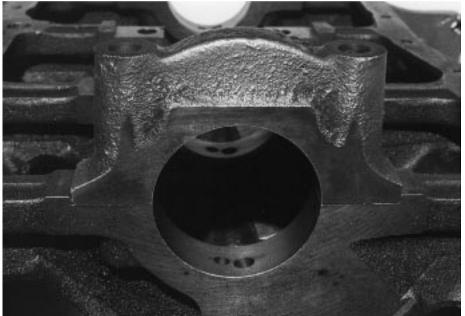
**Main cap sitting in the register of a block. If no effort at all is required to position the cap, the fit is loose. Main caps should need to be tapped into the register.**
