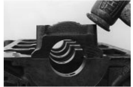
**Main bearing cap being tapped into register by a copper hammer.**
