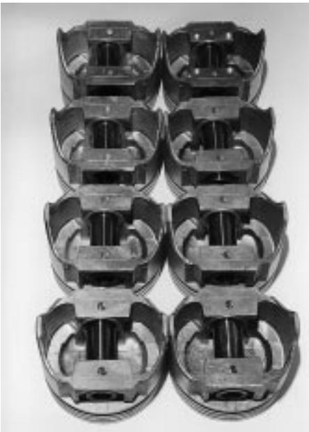
**Typical replacement set of cast pistons.**
