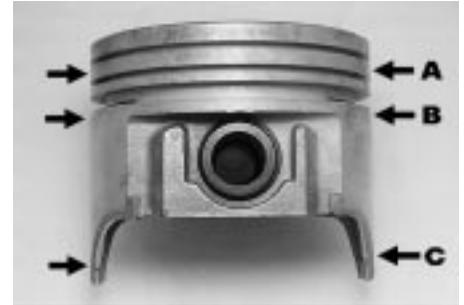
**Dimension "A" is parallel down to the bottom of the oil ring groove and is generally 0.020in less than the bore size. Dimension "B" ( just below the bottom of the oil ring groove) is approximately 0.005in less than the bore size and dimension "C" (the base of the skirt) is usually 0.0015-0.003in less than the bore size. Most stock piston to bore clearances when new are 0.0015-0.002in - the factories make the clearances quite tight and for average street use this is perfectly correct.**
