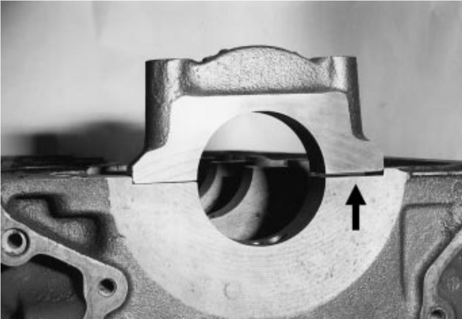
**Main bearing cap sitting on the edge of the block register. The cap should not go into the seat without being “snapped” in.**
