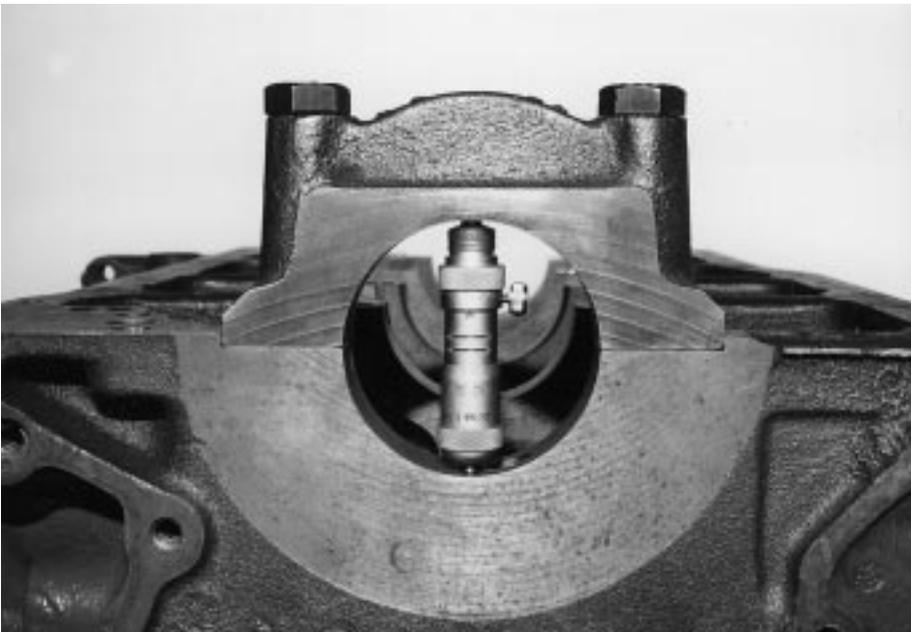
**Main bearing cap properly fitted and an inside micrometer being used to check tunnel size.**
