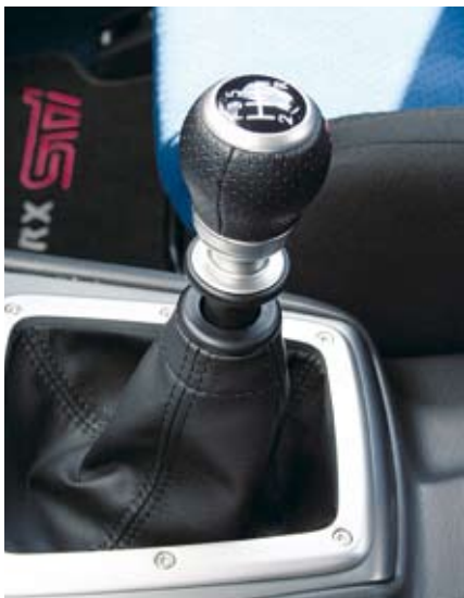
Close-up view of STI gear shift with pull-up reverse ring.
