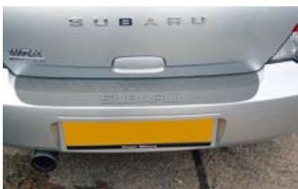
Rubber protector fitted to Impreza WRX.
