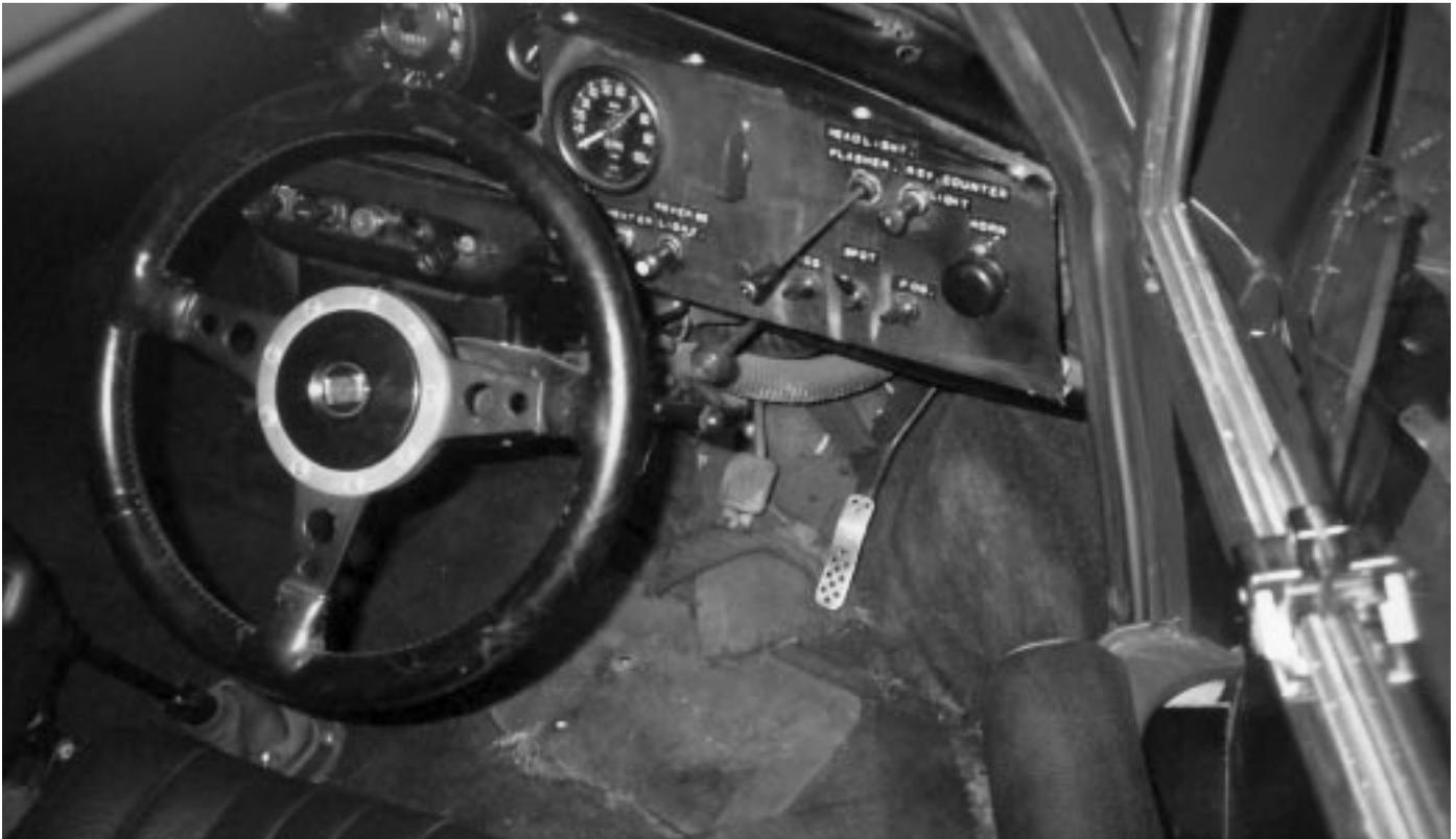
The accelerator pedal with its extension for ease of 'toe and heel' simultaneous brake and throttle operation.
