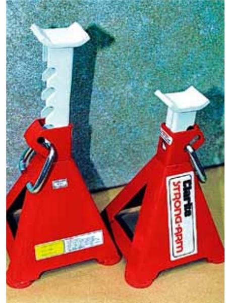
Picture 6. Another must-have is a suitable trolley jack. You'll need to support the vehicle on stands when working beneath it, though. Taller stands with a broader base would be better than those shown.
