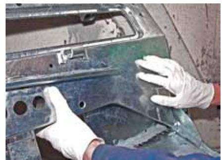
Picture 3. Galvanizing is excellent, of course, but it does have the disadvantage that it almost always buckles the top panel of the bulkhead. Now's the time to put matters right! Rob feels the rippling ...
