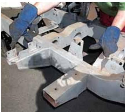
Picture 2. Before Dave at Atkinson-Hadley started work fitting the new bracket, the redundant items had to be removed from the new-old chassis. With his left hand Dave indicates the two high body support brackets that need to be removed, and, with his right, the two outrigger brackets that are in the wrong place.
