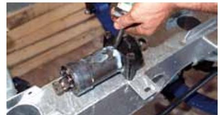
Picture 5. The reason the relay becomes so tight in the chassis is because water and mud get between the two, causing corrosion which then expands the steel and jams the relay in place. If you can keep the moisture out, it will make the relay far easier to remove in future, and will also reduce corrosion on the inside of the chassis. Adrian uses silicon sealer around the top and bottom faces of the relay ...
