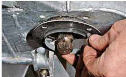
Picture 2. From beneath the front of the chassis, remove the four bolts and spring washers securing the relay lower flange plate to the chassis.
