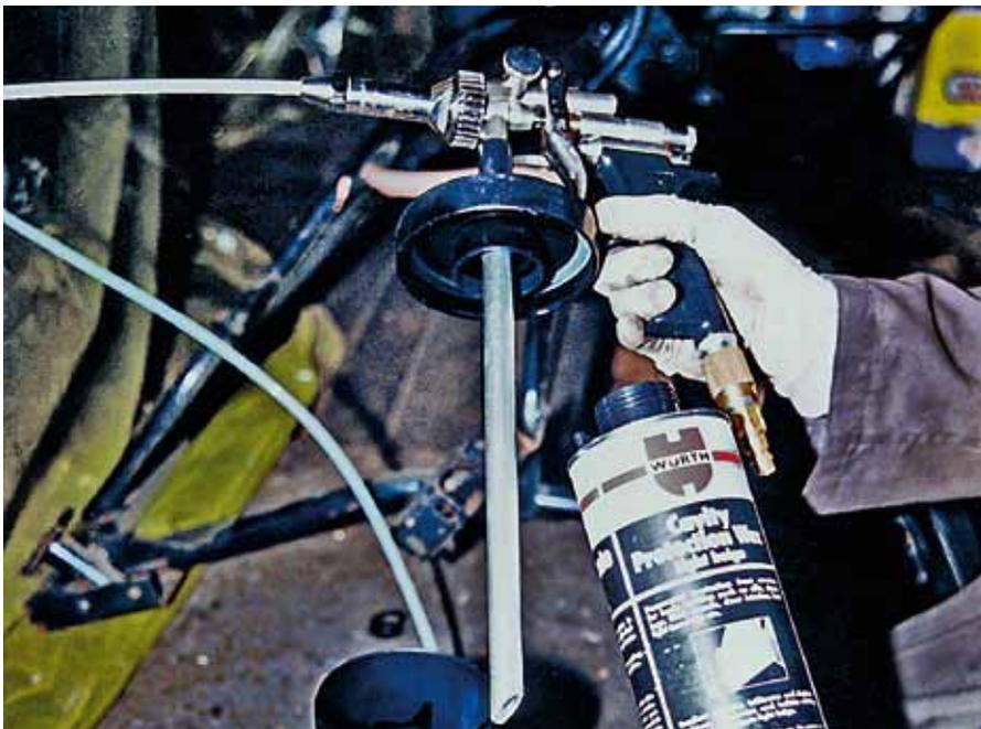
Picture 5. You could always hire a compressor when you need it for specific jobs, such as injecting rustproofing fluid.
