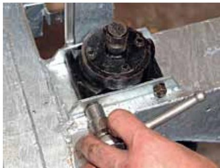
Picture 3. Remove the nuts and spring washers from the two bolts (see picture 1, item 8) securing the relay to the chassis.
