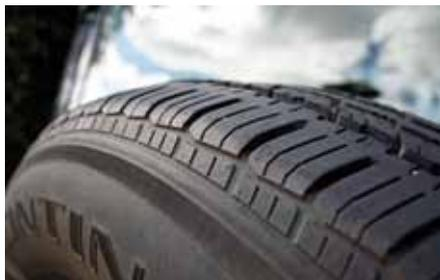
**Door-mounted spare tyres receive higher levels of UV, and can perish even faster than the ones on the road. Spare wheel covers can help.**
