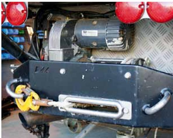
This rear winch has a solid fairlead, synthetic rope, and substantial recovery eyes securely welded-on – ideal for doubling up the rope via a pulley.
