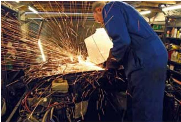
It's a brave man that cuts up his family car in order to build a dream. Here, the bulkhead is trimmed to fit the engine. (Courtesy F Buxton)
