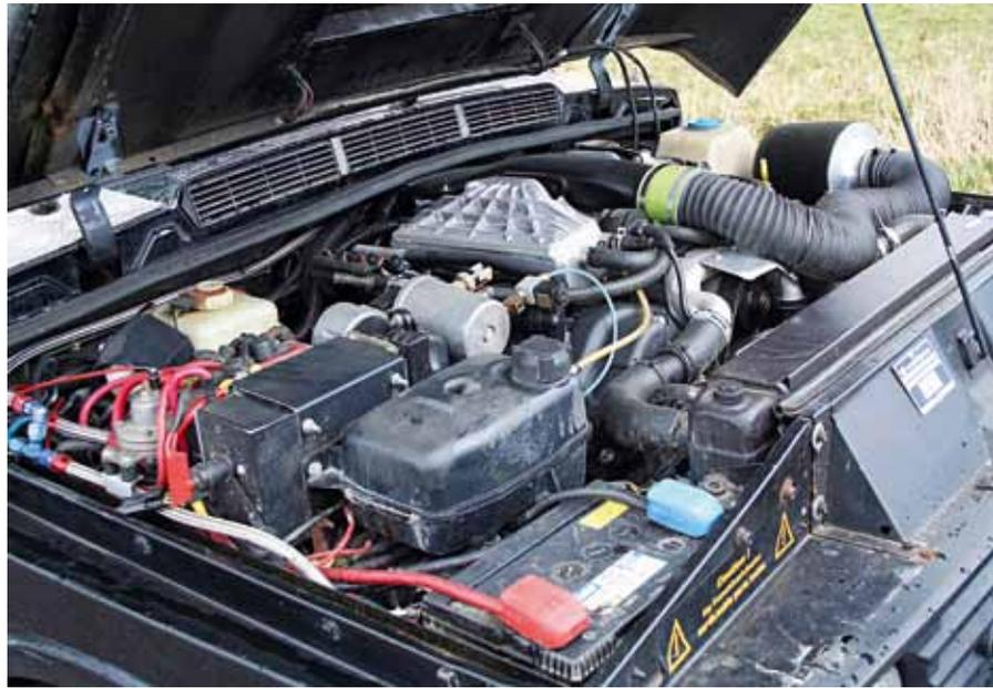
A full engine bay; supercharger, LPG system, split charge, winch controls, and ARB air pump all sit neatly together.
