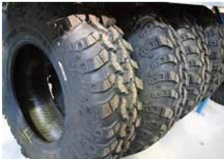
The tyre carcass has a substantial influence on performance; softer ones can have better grip at the expense of resistance to damage and punctures.
