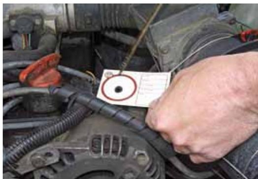
**The oil condition can be tested on special paper cards that let the drop of oil spread out into its component parts.**
