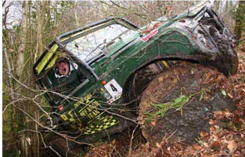
This tyre has become blocked with sticky yet slippery mud, resulting in the winch being needed. (Courtesy Devon 4x4)
