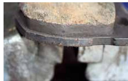
**Look closely and the tiny crack between the friction material and the metal backing on this old brake pad is visible. The other pad on this calliper completely lost its friction material during an emergency stop.**
