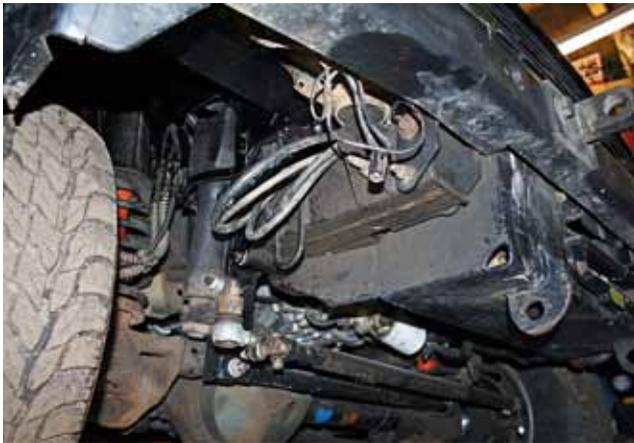
Engine ancillaries dictated that the steering box had to move outboard of the chassis. The solution is a P38a box and custom link rods.
