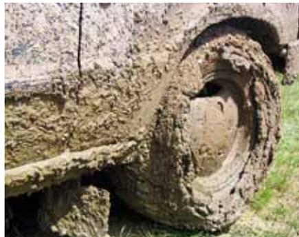
The chevron tread pattern has forced the sticky mud out into a band at the side of the tyre.
