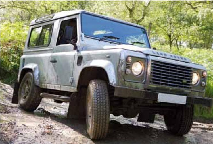
A narrower tyre can outperform a wide tyre where it has to sink through surface mud to reach hard ground. (Courtesy Land Rover)
