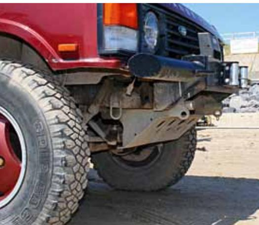
The winch here is mounted behind the bumper, which reduces front protrusion, but means the grille must be modified to fit it.
