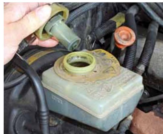
**Brake fluid can turn dark grey as it ages. If it looks this black, the car is at serious risk from brake fade under heavy braking.**
