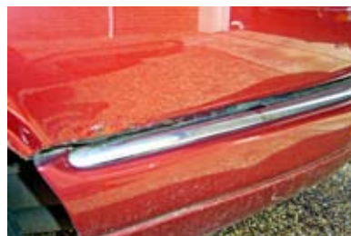
Corroded mounts let bumper hang.
