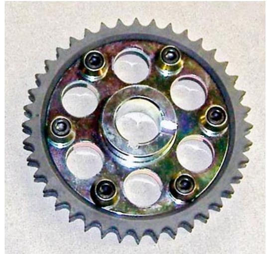
**3-5 An MGC vernier timing sprocket bolts to the camshaft, of course, which reminds me to mention that new camshaft blanks are not now being produced. As a result, you'll need a good, straight camshaft to trade-in if/when you seek an uprated one.**
