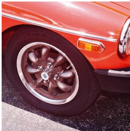
10-5 These are the more usual bolt-on Minilite wheels but this time finished in 'Slate.' The polished rims require some additional maintenance in that without care their surface will corrode.
