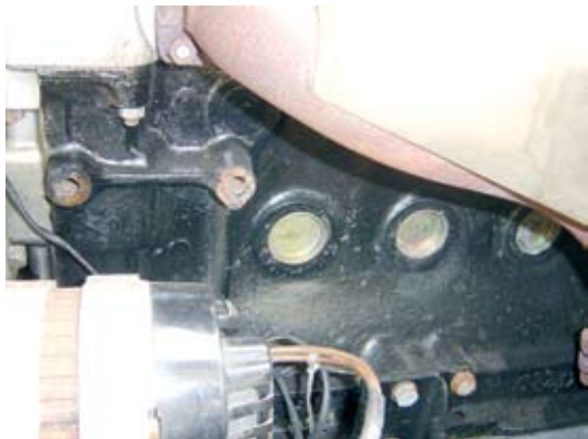
New core plugs. A good sign.
