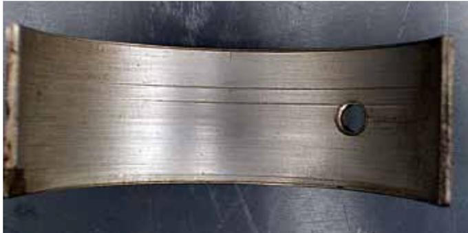
32. This connecting rod (big-end) bearing has been scored by debris in the oil: consequently, oil pressure will be reduced.
