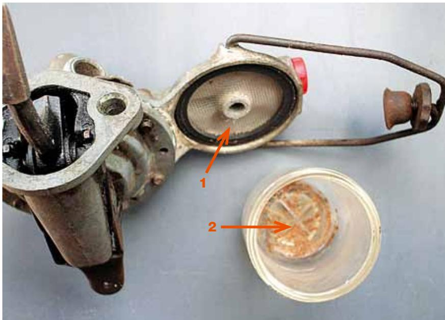
47. Clean the gauze filter (arrow 1) in the top of the pump, above the sediment bowl. Also remove any sediment (arrow 2) that may have collected in the bowl.
