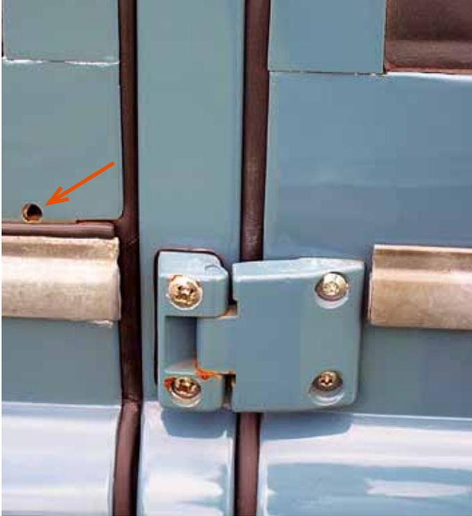
**116. Door hinges should be adjusted to give even gaps around the door seals. Notice the water vent hole on the left (arrowed).**
