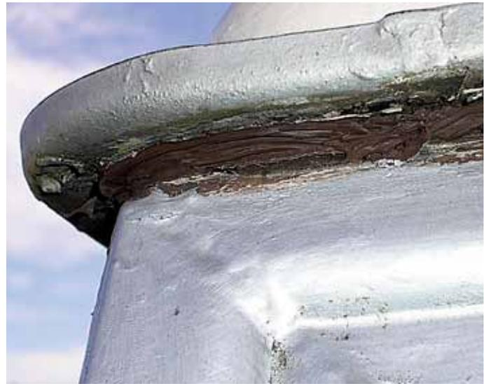
**117. If you don't ever fold your Land Rover's windscreen flat, then you could seal any leak with non-hardening sealant, as here.**
