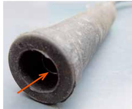
**1. Metal connectors are deeply embedded in the plug leads. Check them for corrosion and for a positive 'click' when refitting.**
