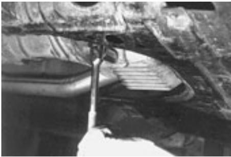
3/3b ... loosen the oil pan drain plug ...
