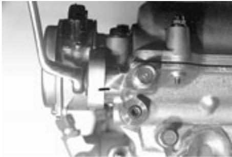
9/131 Align marks and tighten bolt.
