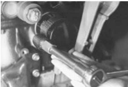
3/4 Use a strap wrench to loosen filter ...
