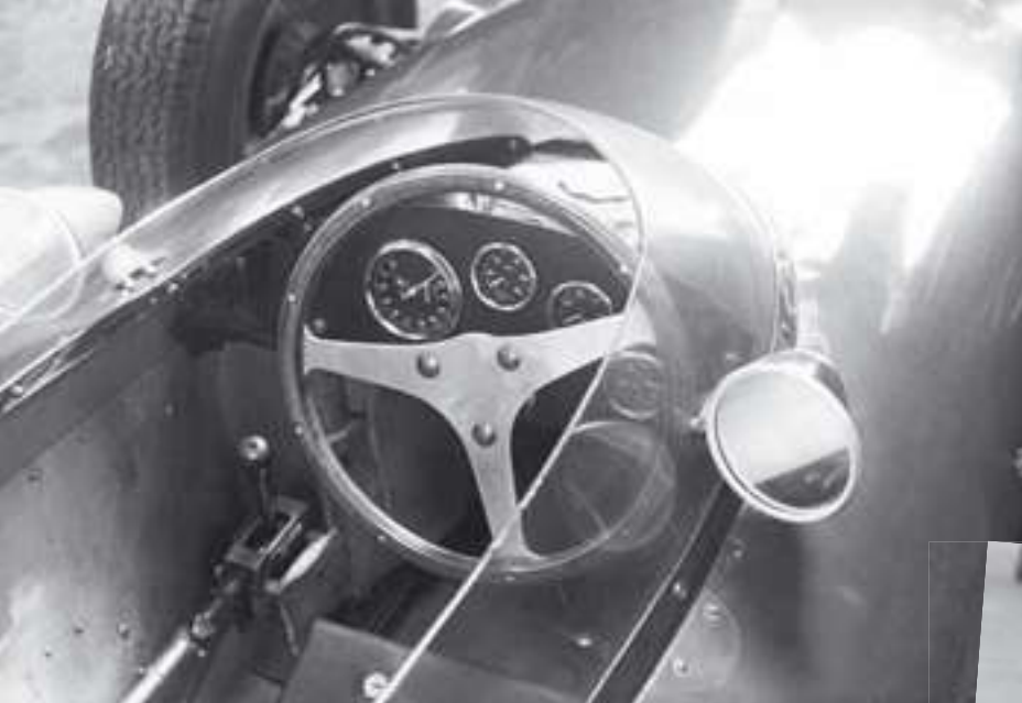
The instrument panel on a P57 BRM in racing trim. Left to right: rev counter, oil pressure, water temperature and fuel pressure gauges.
