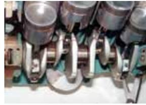
The bottom end main and big end bearings require much work to rectify serious wear.
