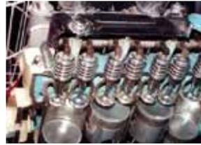
The rocker shaft (across the top of the picture) and rockers wear and, subsequently, rattle.
