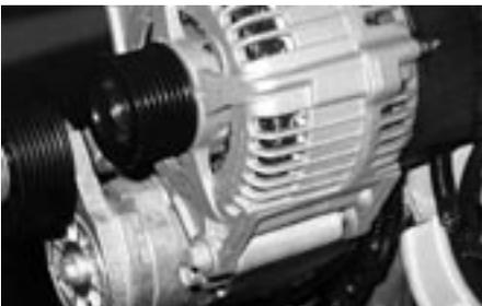
**13-1-3 A modern high amperage alternator with internal fan. Note the different fan/drive belt (no more 'V' belts) which gives food for thought insofar as water pump and crankshaft pulley shapes are concerned.**
