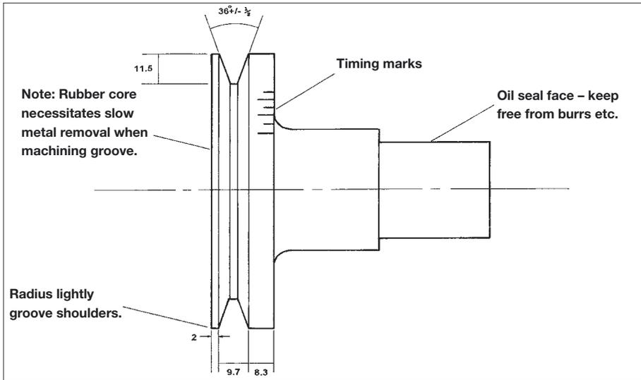
**D2-1 Machining detail for fanbelt groove in SD1 crankshaft pulley.**
