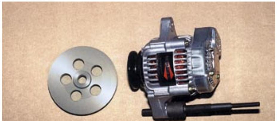
**13-1-5 A neat Cambridge Motor Sport 45 amp alternator conversion kit. Also in shot is the large aluminium pulley that you will need to drop alternator (any alternator) rpm down to something more practical when the engine is running at the high rpm expected in competition. Note the special single mounting pivot supplied with the kit.**
