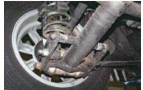
**8-3-12-2** A closer view of the unnecessarily altered bottom damper mounting. The spacing washers seen very clearly here substitute for the original space taken up by properly positioned dampers.
