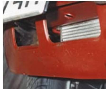
**5-3-3** The vented front valance fitted as standard to later chrome-bumper MGBs. I initially fitted this to my GT V8 conversion, but changed to an ST spoiler in the interests of additional air flow through the radiator and better front-end stability.
