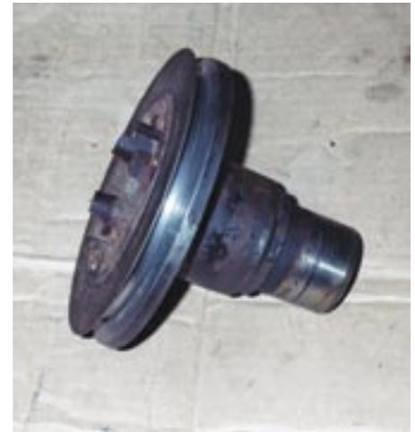
**2-2-4 Later Rover front pulleys may consist of differing components but should still provide ...**
