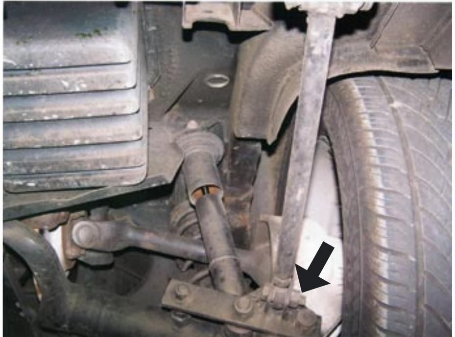
**8-3-12-1** This view will differ from the usual Jaguar rear mounting arrangement because the dampers have been moved outboard by 3in (75mm). However, the rear radius arm mounting will be as you expect to find it. The arrowed bushes need replacing with polyurethane ones and, ideally in my view, the arm needs cutting and re-welding here to crank the front end of the arm over towards the centre of the car in order that the front pivot is axially in line with the inner wishbone pivot.
