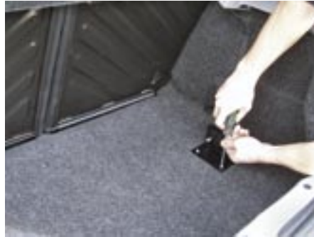
The pipe has to be carefully routed from the nitrous cylinder to the nitrous solenoid.
