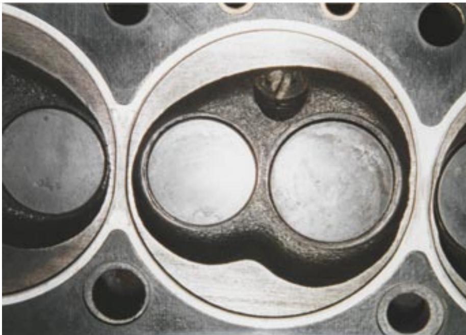
Standard MG Metro Turbo cylinder head combustion chamber and valves. The standard 1275cc engine's combustion chamber is almost exactly the same shape.
