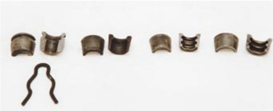
**Collets/keepers/split locks: early style ones for 850cc, 998cc and 1098cc engines, extreme left; 1275cc single groove ones (which were later universally used on all engines up until A+ engines came out) centre left. A+ 998cc and 1275cc triple groove ones for standard diameter valve stems, centre right; A+ MG Metro Turbo, triple groove, large diameter valve stems, extreme right.**
