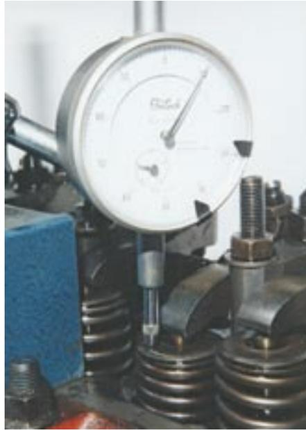
Valve is at full lift. Zero the dial and then count back as the valve returns to its seat.
