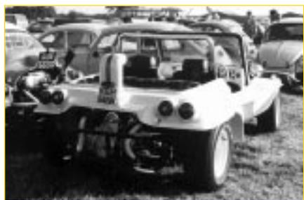
The tall periscope could be used to increase the flow of cooling air to the VW engine, or the base could be adapted to mount a Formula-1 style rear wing (also available from the manufacturers). The Albar "S" buggy used twin round rear lamp units.
