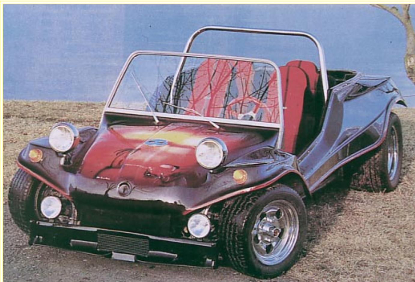
The Albar "ES," with unitary bodyshell laminated in flame-retardant resin, and traditional alloy windshield frame, was a cheaper kit option. The design had noticeably lower sides to the body waistline, but still fitted the stock VW floorpan. The kit was also made in Britain, though few were sold.
