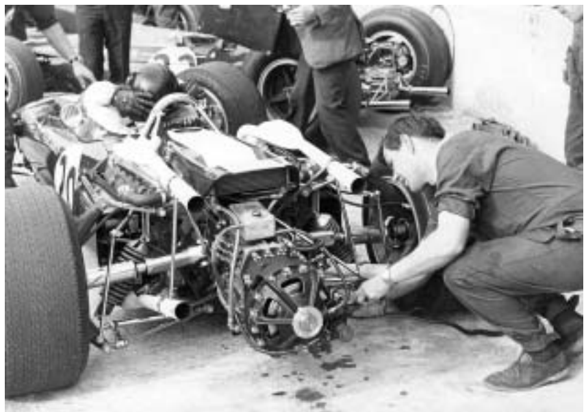
The complicated, unreliable and bulky BRM H16 engine. Installed in the back of a Lotus 43, it scored its only Grand Prix victory with Clark behind the wheel at Watkins Glen in 1966. (Goddard Picture Library)
