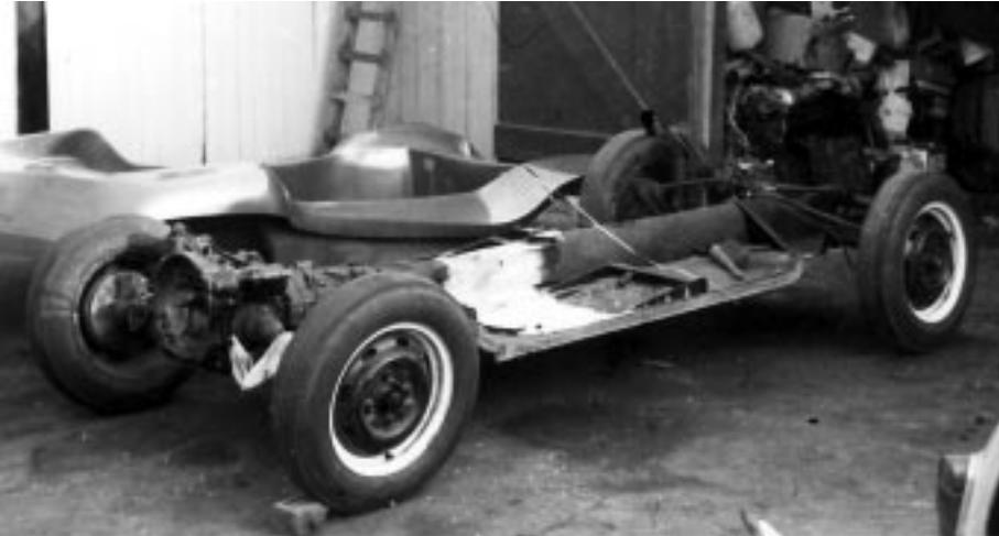
A Beetle chassis prepared to accept a dune buggy bodyshell. The simplicity and strength of the rolling chassis design has made it ideal for building buggies. (Courtesy John Jackson).
