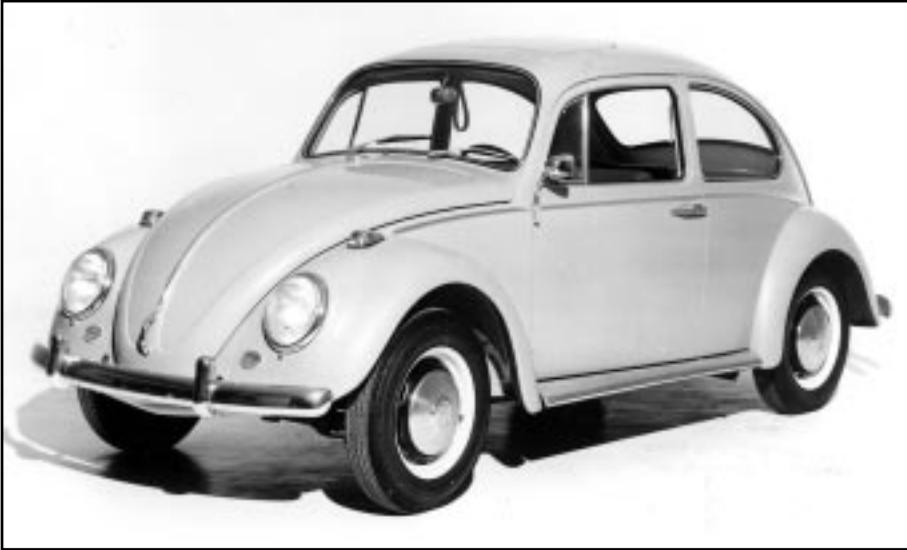
The classic 1960s Beetle with king and linkpin front suspension, and swing-axle rear suspension. Many of the components can now be upgraded with high performance parts. (Courtesy Beaulieu Picture Library).
