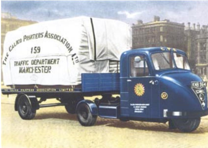
A familiar sight at docks and railway stations around the country was the Scammell Scarab mechanical horse. Depicted in Manchester around 1949, these three-wheeled tractor units were highly manoeuvrable, a requirement when working at ports and on railway station platforms. (Author's collection)
