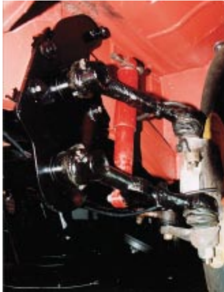
Harry Harpic's modified torsion beam with welded steel endplates to adapt late ball joint beams into earlier Buses. (Courtesy Paul Knight)
