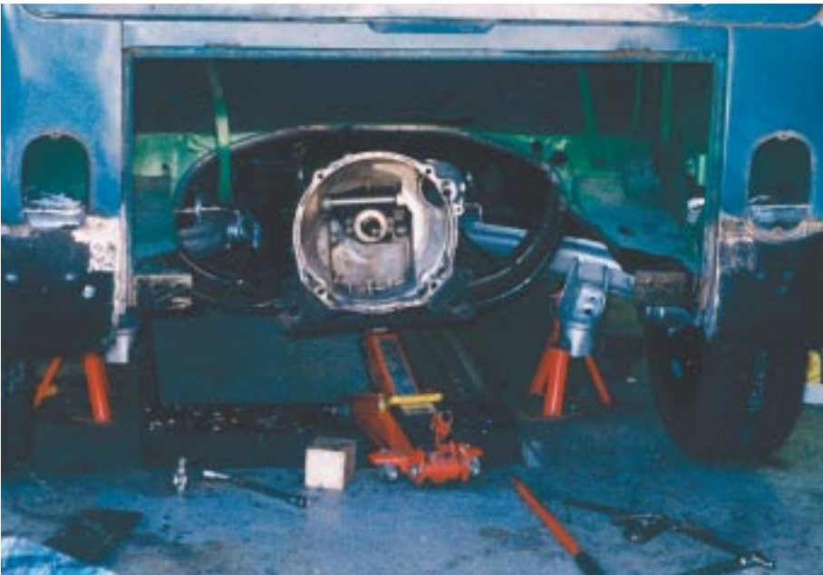
Trial fit of all IRS components into early Bus before welding brackets in place. (Courtesy Paul Utting)
