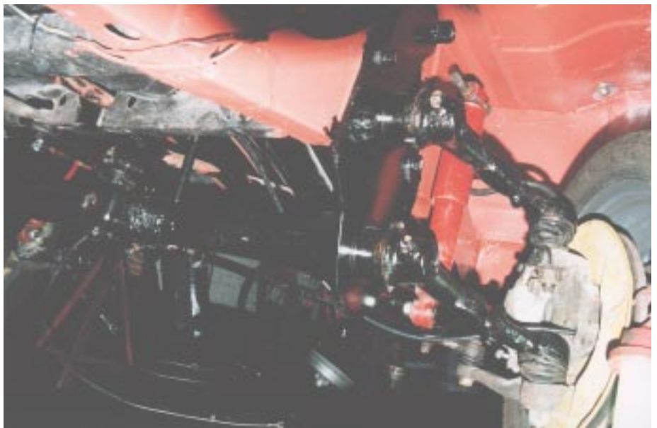
The modified beam can also be narrowed to prevent front inner wheel arch modification when lowering a Bus. (Courtesy Paul Knight)
