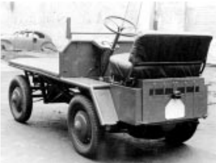
Plattenwagens were crude VW-based transporters used to move components around the VW factory. (Courtesy Walter Bach)
