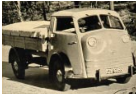
Front-wheel drive commercial vehicle, the Tempo Matador, used the air-cooled engine from a VW Beetle.
