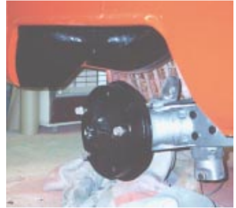
A-arms fitted and drums in place on Split Screen van. (Courtesy Paul Utting)
