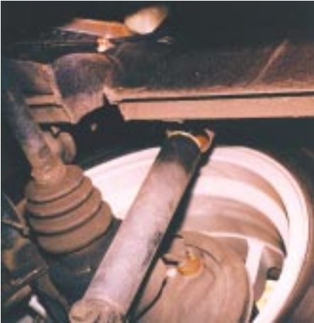
Chassis channelled to clear IRS axles for road use – here shown on a 1971 Crew Cab Bus. (Courtesy Simon Glen)
