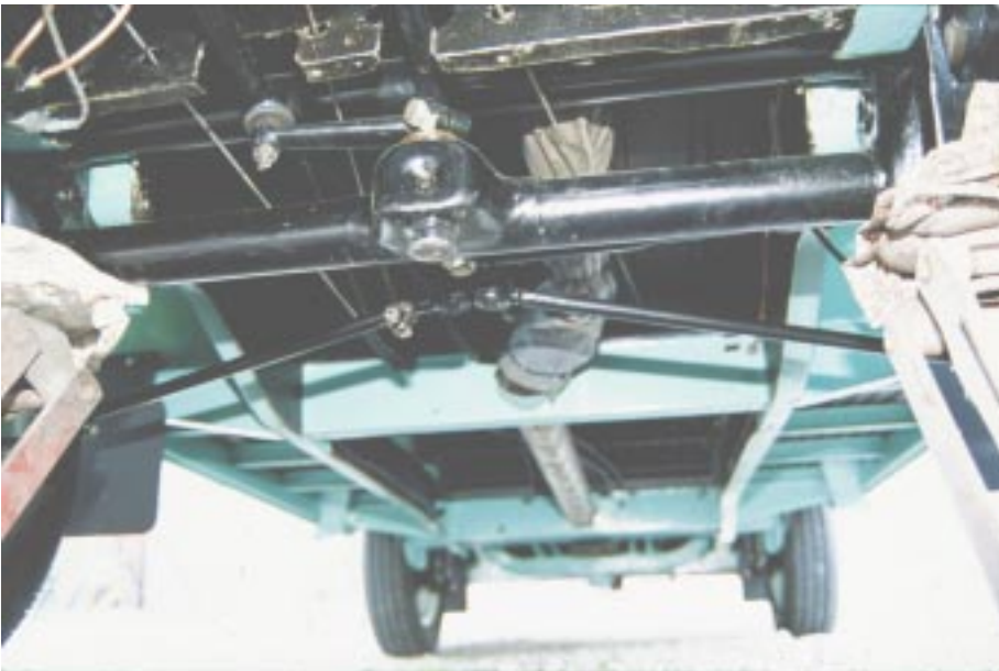
The underside of a fully restored 1963 Split-screen Bus. The front suspension is a very strong unit, with steering pivots provided by king and linkpins. (Courtesy Alex Leighton)
