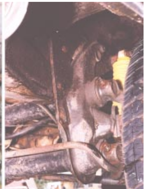
A thick steel plate is normally welded to the axle beam flange to 'lift' the body about 4in from the suspension. (Courtesy Simon Glen)
