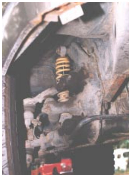
A thick steel plate is normally welded to the axle beam flange to 'lift' the body about 4in from the suspension. (Courtesy Simon Glen)
