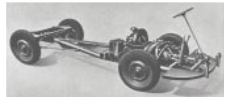
View of the Tempo Matador chassis, steering and drivetrain.
