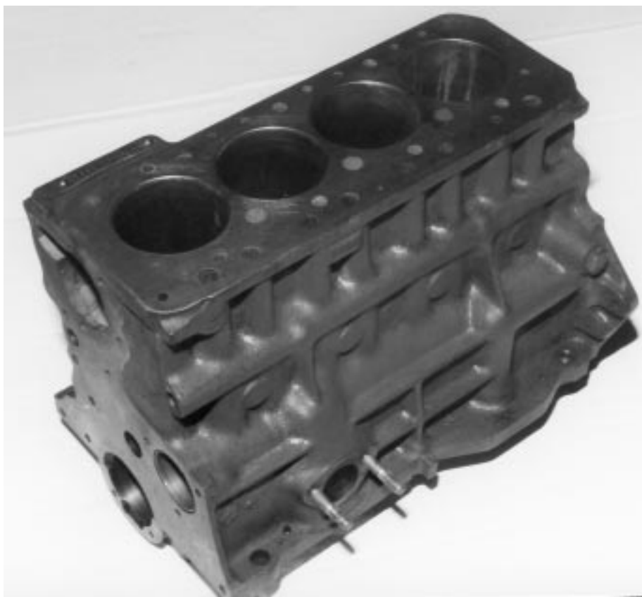
1275cc A+ cylinder block. Note the strengthening ribs.
