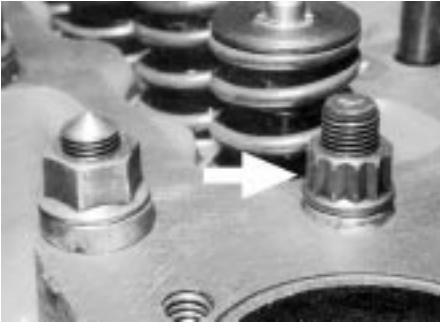
Connecting rod nut used on extra stud. Note that because this head has been planed by 0.120in/3.0mm, thick washers are placed under the nuts to compensate.
