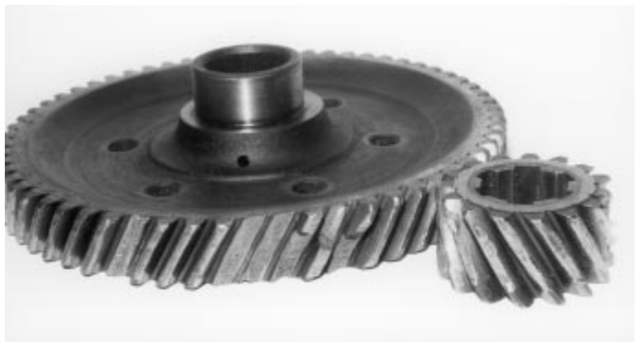
Standard type of final drive with broken teeth.
