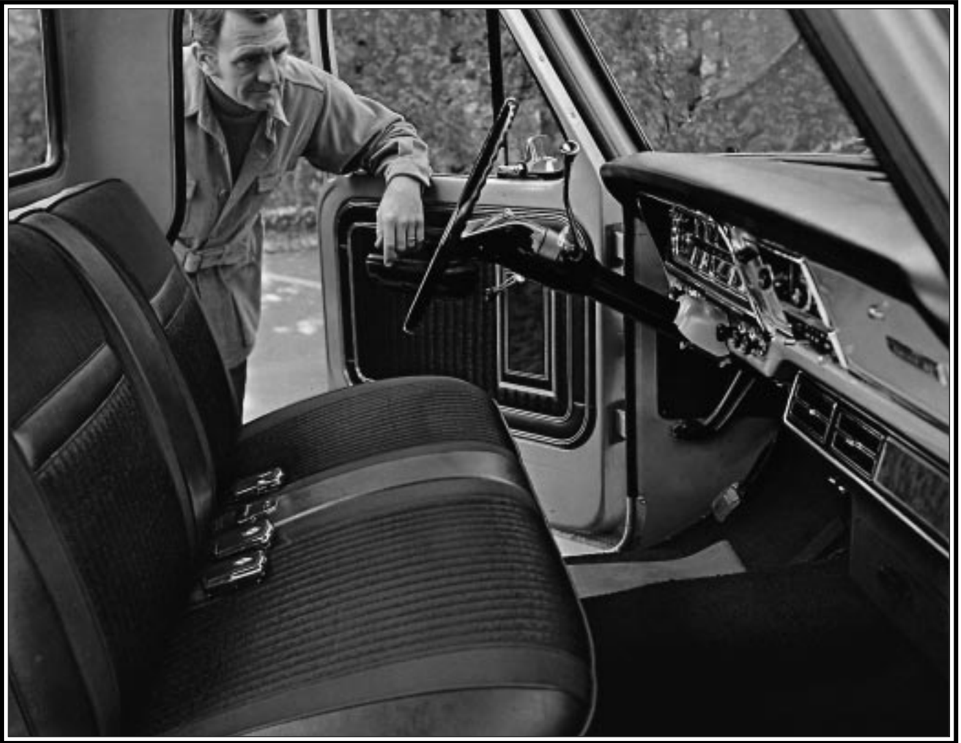
Changes made in the 1971 Ranger XLT interior included a repositioned woodtone door panel and revised upholstery pattern. (Courtesy Ford Motor Company)
